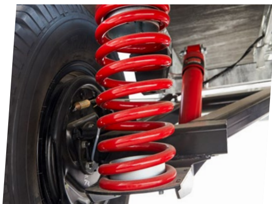
Australian engineered and manufactured JTECH 2.0 trailing-arm suspension is compact in size, durable and reacts better to road undulations.*
