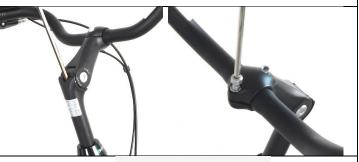
5. Insert the Saddle column into the bike, making sure to orient the saddle and tighten the saddle with the appropriate device on the frame as shown in the image on the right.
