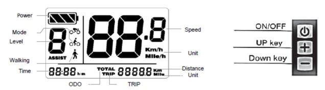
**ON/OFF** - Long press On/Off to start display. Long press On/Off again to switch off. Display off automatically after no any operation on vehicle for ten minutes (default).
