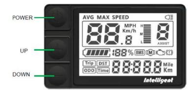
**ON/OFF** - Press and hold Power button for 1.5 second can turn on/off the display. The Display can automatically shut down when there is no operate  $\alpha$  ride for X minutes (X could be  $0 \sim 9$ ).
