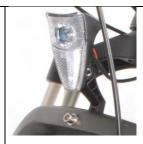
4. Remove the front plate located on the handlebar column.
