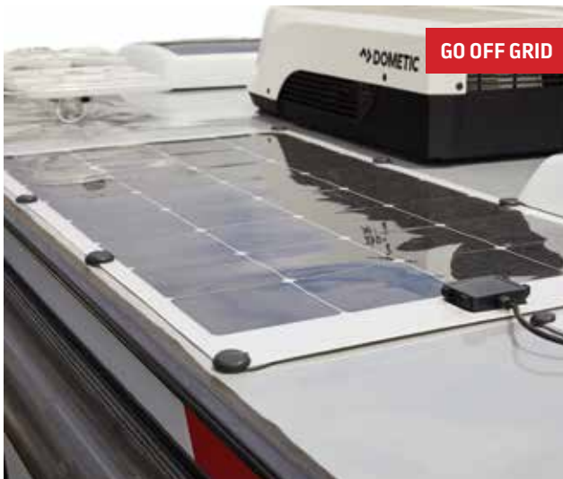
3x 150 W solar panels for power supply for extended trips away from it all.
